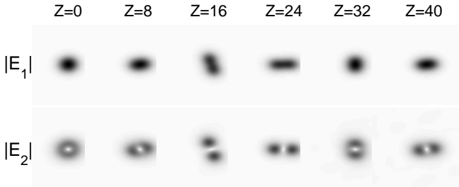
FIG. 7. Break-up of an unstable vortex soliton into a rotating dipole soliton under the perturbation (66)–(67) with s = 0.5 , \lambda = 0.45 , and \alpha = 0.05 .
